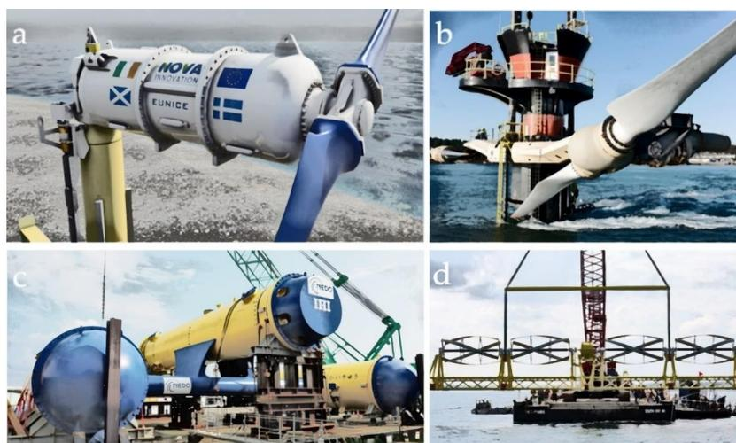
**Figure 4.** The hydrokinetic devices selected for the techno-economic analysis: (a) NOVA M100-D turbine, with permission of [51]. (b) Sea Gen turbine, adapted from [52]. (c) Kairyu turbine, adapted from [49]. (d) TidGen turbine, with permission of [50].
